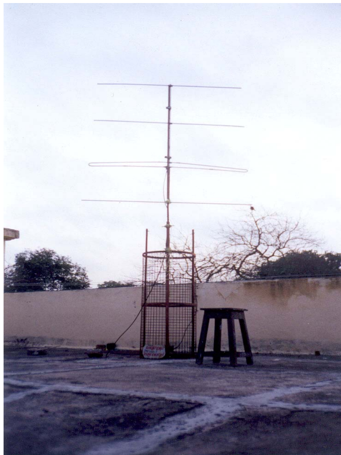
Figure 9: The 3-element Yagi Antenna of frequency 91 MHz.
