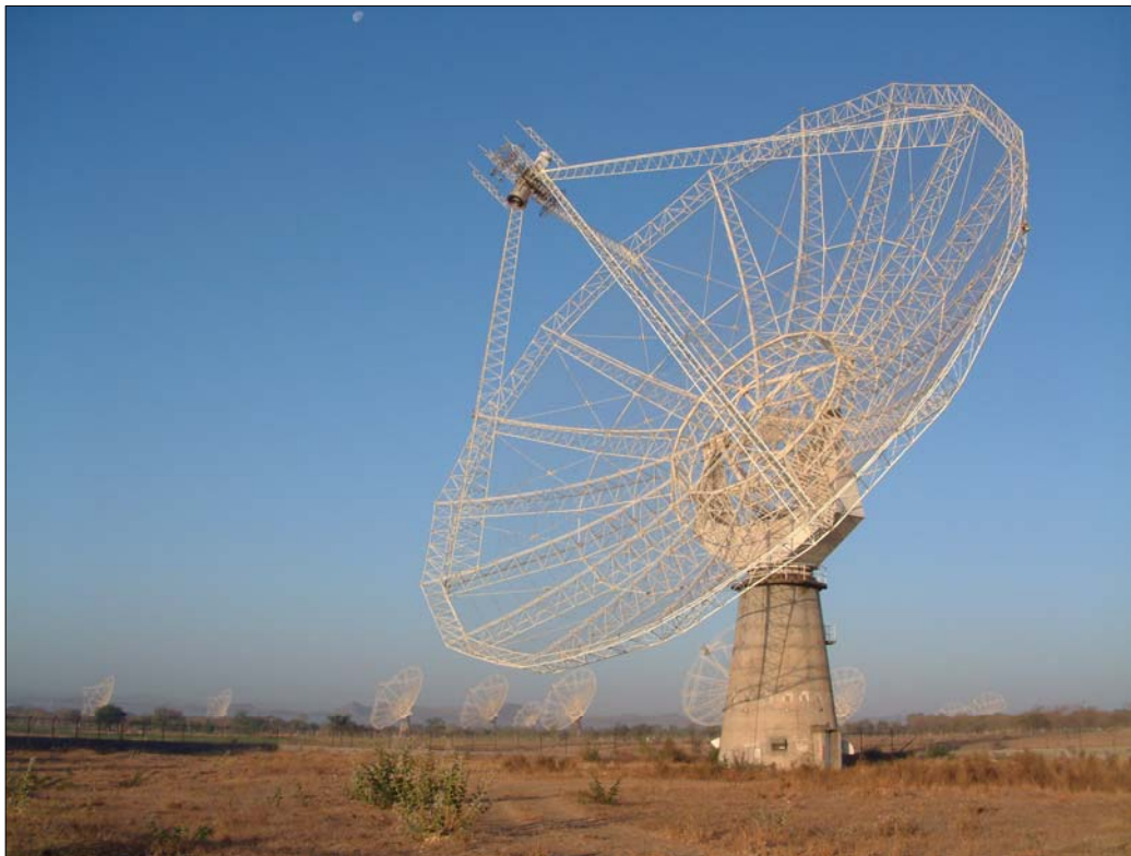
Figure 18: A close view of one of the thirty 45 m diameter fully steerable parabolic dishes of the Giant Metre Wavelength Telescope located at Khodad, near Pune, in western India. A few dishes of the central array of the GMRT are also visible in this picture.
